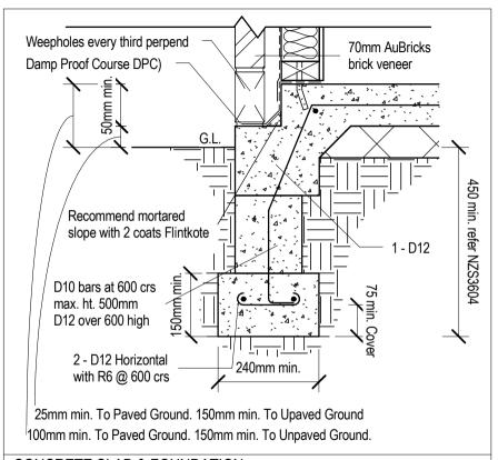
CONCRETE SLAB & FOUNDATION OPTION 1 - MIN. REQIRED FOR 1 & 2 STOREY
